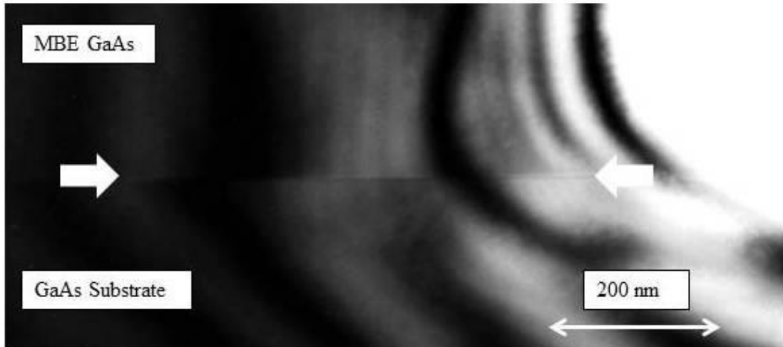
Figure 4-15: BF micrograph of MBE GaAs on (100) LEC-GaAs substrate. The interface is relatively perfect and there are very few features to see. The interface is indicated by two arrows.
