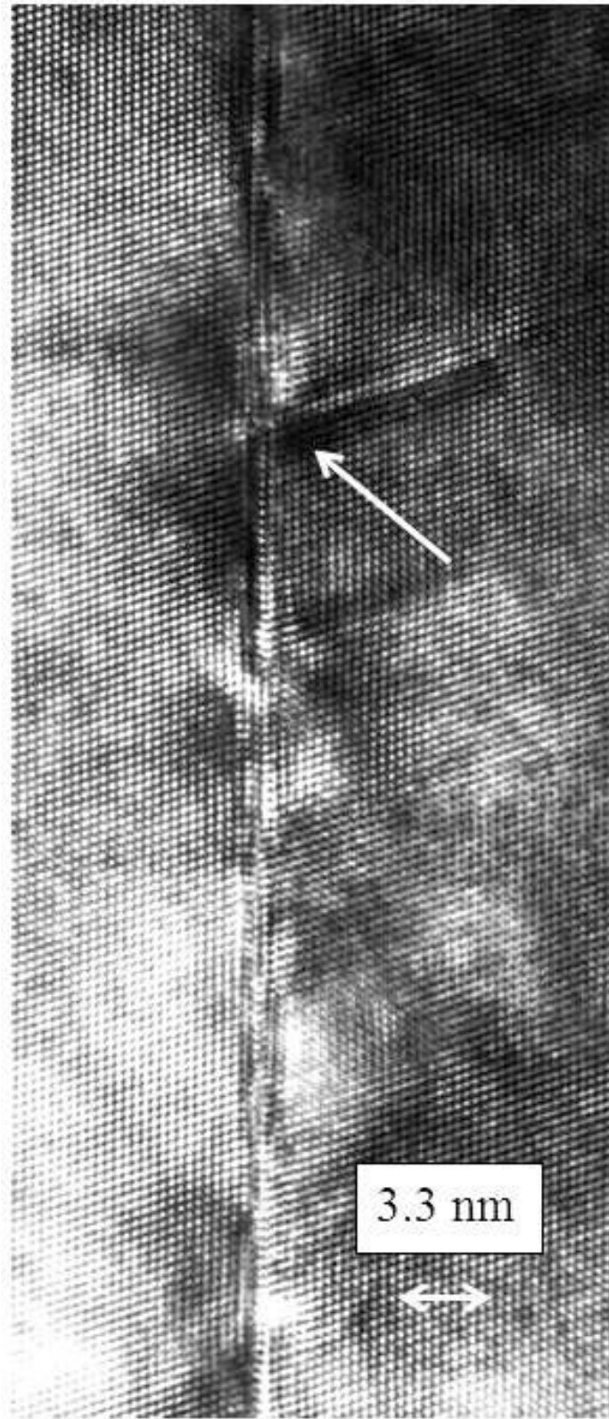
Figure 4-13: HRTEM of extended microdefects in the LEC-GaAs crystal with defects on multiple (111) planes, which may have formed because of the merging of multiple microdefects. It also contains a locked dislocation (arrowed). Similar locked dislocation was described for the CdTe in Chapter 1, figure 1-54.
