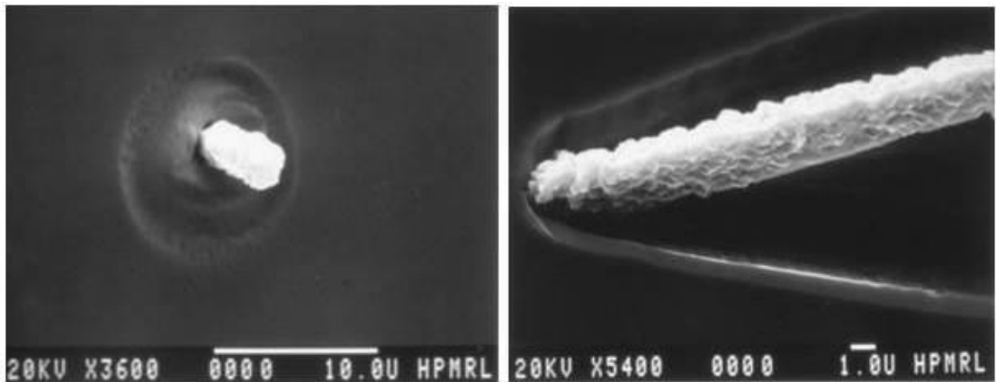
Figure 4-37: SEM micrograph of shorter GaAs whiskers showing more detail of its morphology. The image on the left clearly shows that the base of the whisker is the same oval defects that were being seen earlier, and that whiskers appear to be the outgrowth of the white balls seen inside of the oval defects.
