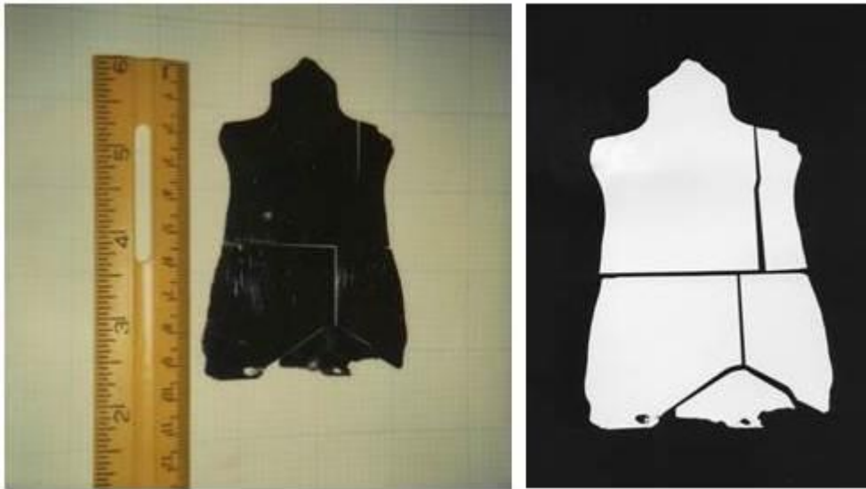
Figure 4-5: Undoped GaAs ingot H155, cut length-wise across the boule to obtain wafers. The image on the right is the same wafers shown on the left, taken with higher contrast to show the different wafers that were cut.
