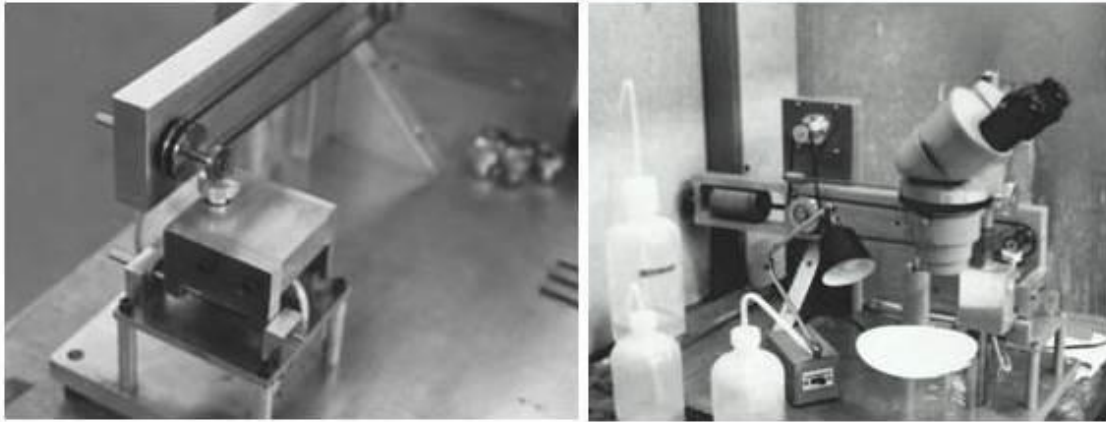
Figure 1-15: Left, a close-up detail of the dimpler grinding wheel and the turntable. Right photo shows the microscope used to monitor the progress of dimpling the specimen.
