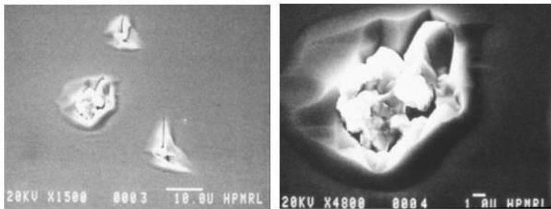
Figure 4-33: SEM micrographs of irregularly shaped “oval” defects. They also contained white particles inside, but often they were also irregularly shaped and polycrystalline. They have the typical appearance of external “impact” defects, where a particle fell on the substrate and film grew around it.
