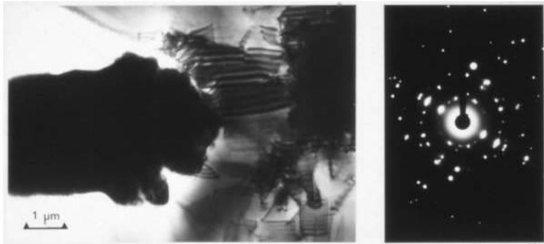
Figure 4-46: A BF HV-TEM image at the base of a whisker showing a high density of defects at the base, and polycrystalline characteristics of the base material.
