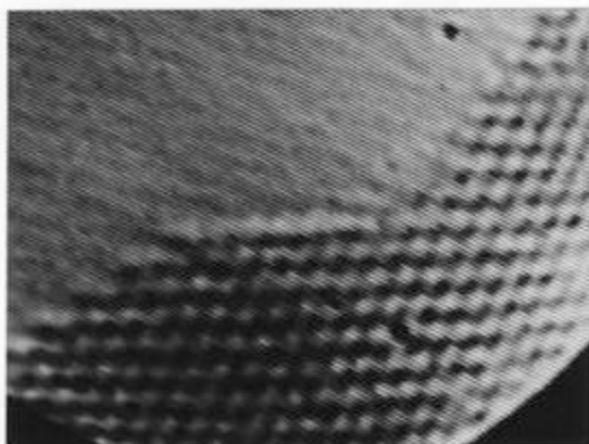
Figure 1-82: Video image from the edge of the specimen where surface rearrangement is taking place. The images are digitally processed and enhanced.
