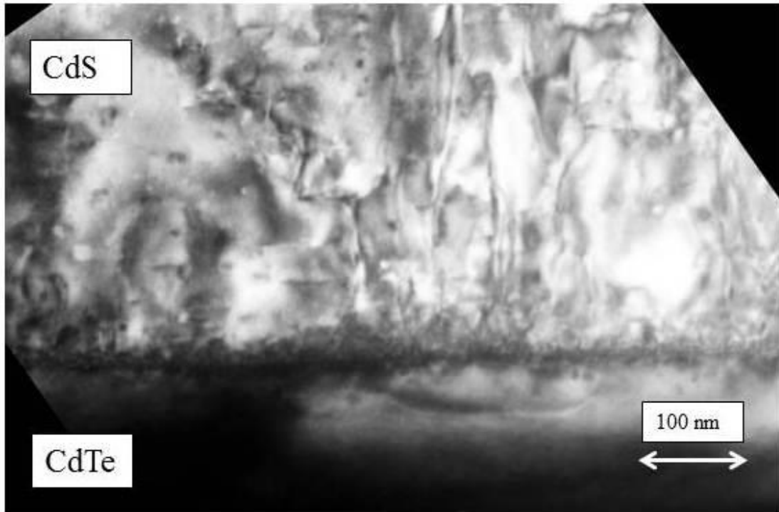
Figure 3-46: BF micrograph of the CdS/CdTe interface. CdS has a large area where it is single crystalline, but in some areas (center), there are subgrain-like structures, which are at slightly different orientation with respect to the neighboring regions.
