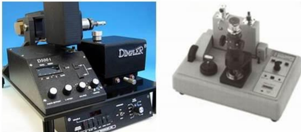
Figure 1-20: Left, a commercial Dimpler ® tool built by the VCR group [1-38] by Vince Carlino who licensed the design from HP Laboratories and Tom Cass. Right, a Gatan Dimple Grinder [1-37] with a simple and compact design.
